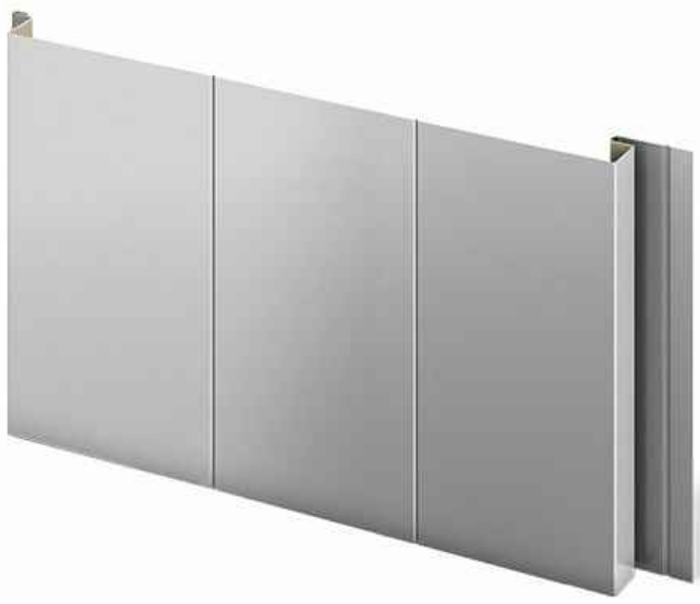
BLOCK 45B METAL PANEL SYSTEM 2 BERRIDGE L-PANEL SIZE: 24 GAUGE STEEL COVERAGE: 11 5/8" FINISH: BLACK, SMOOTH FASTENER: CONCEALED BRAND: BERRIDGE
