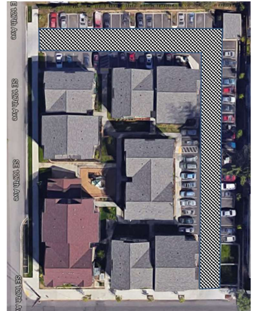
Site with 30 percent of area used for surface parking. The hatched area shows the maximum 15 percent of site area that could be paved with asphalt.
