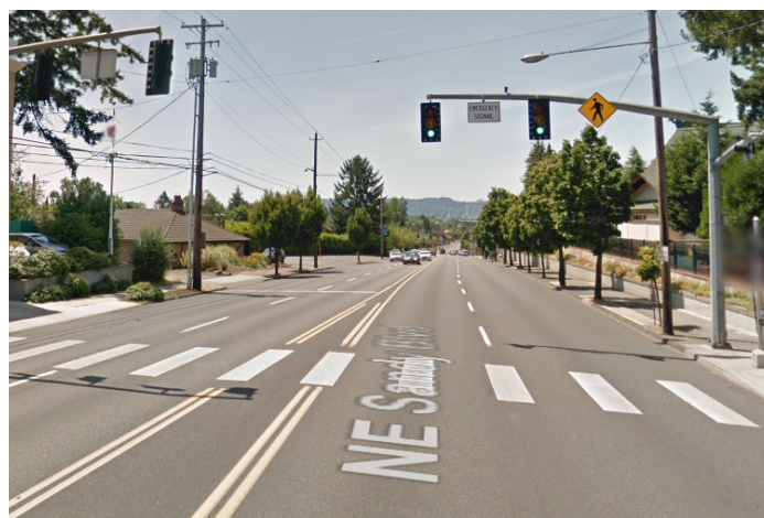
A fire signal was converted to serve as a pedestrian crossing on NE Sandy
