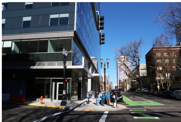
Curb extensions at signalized intersections can increase visibility of pedestrians attempting to cross the street. They also help set back vehicle parking to improve sight lines.
