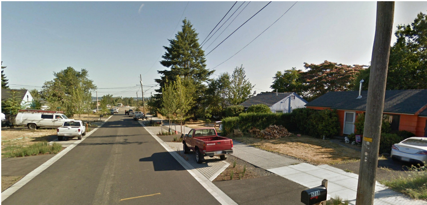
NE 72nd Ave in Northeast Portland provides a separated walkway with integrated landscaping, stormwater facilities and on-street parking.
