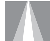
SPT - Spot Beam angle 15° Field angle 39° Spacing criteria 0.2
