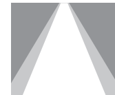
WFL - Wide Flood Beam angle 45° Field angle 62° Spacing criteria 0.8
