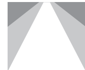
WFL - Wide Flood Beam angle 55° Field angle 104° Spacing criteria 0.8
