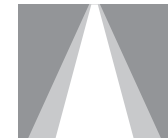
FLD - Flood Beam angle 30° Field angle 49° Spacing criteria 0.5
