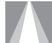
NFL - Narrow Flood Beam angle 25° Field angle 48° Spacing criteria 0.4
