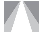
FLD - Flood Beam angle 35° Field angle 67° Spacing criteria 0.6
