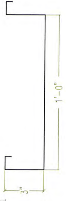
9 24GA HIGH SEAM ROOF PANEL SCALE: NTS
