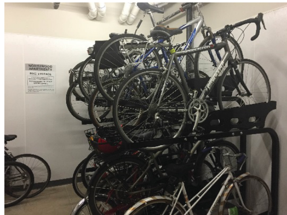
Double Decker rack – no lift assist. Room for 12 bicycles.
