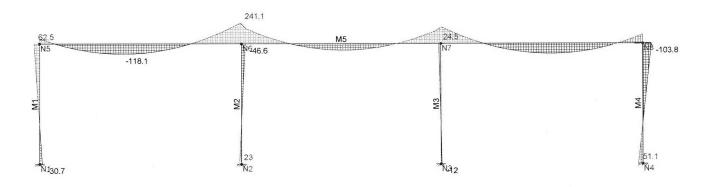
Results for LC 12, Gravity only (Static N1) Member z Bending Moments (k-ft)
