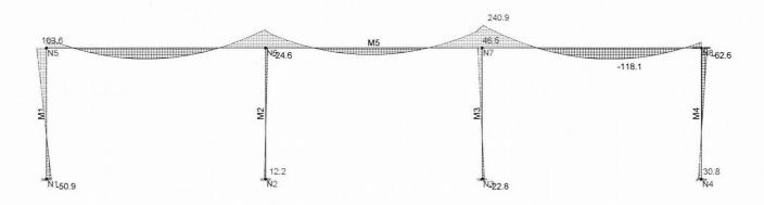
Results for LC 15, Gravity only (Static N4) Member z Bending Moments (k-ft)
