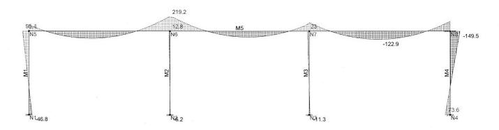
Results for LC 14, Gravity only (Static N3) Member z Bending Moments (k-ft)
