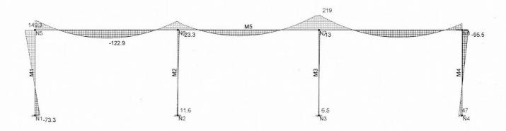
Results for LC 13, Gravity only (Static N2) Member z Bending Moments (k-ft)
