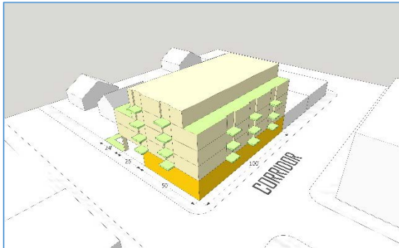
The diagrams above show an example of the massing of development allowances in the CM3 zone. The left diagram shows the maximum base development allowance; the right diagram shows the maximum allowance with bonus.
