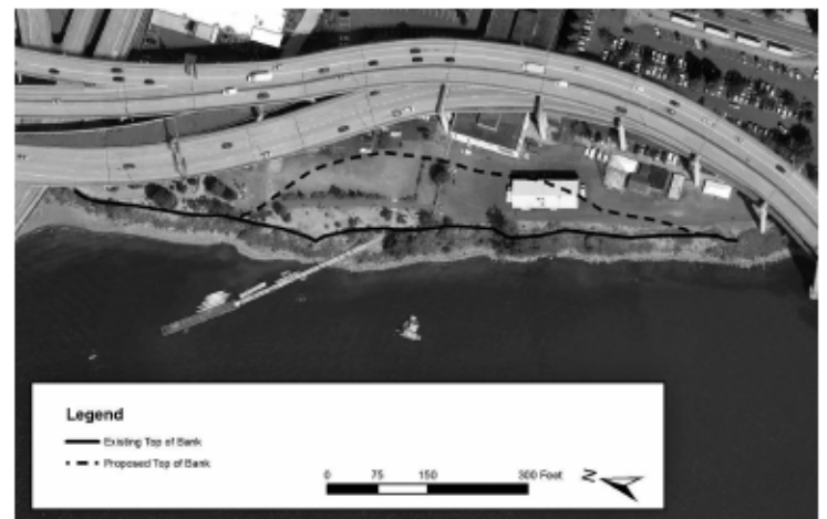
Figure 4: Existing and proposed (Concept 1) top of bank line showing extent of potential bank layback at the site
