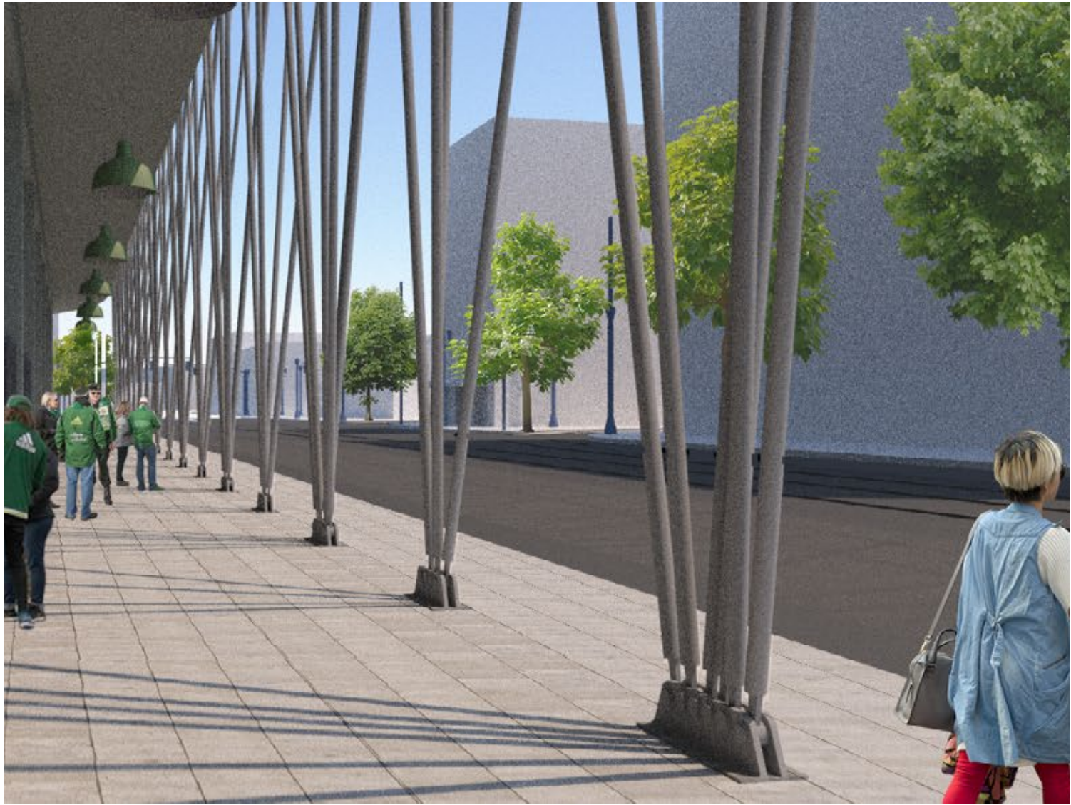
ELEVATED BASE CONNECTION WITH CANE DETECTION ELEMENT
