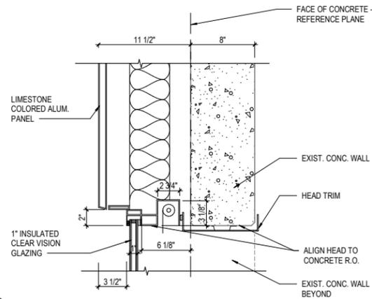
**E** WALL TYPE "B" - HEAD AT PUNCHED OPENING
