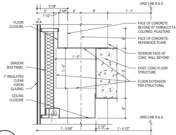
**E** WALL TYPE "C" - FLOOR SLAB SHADOW BOX
