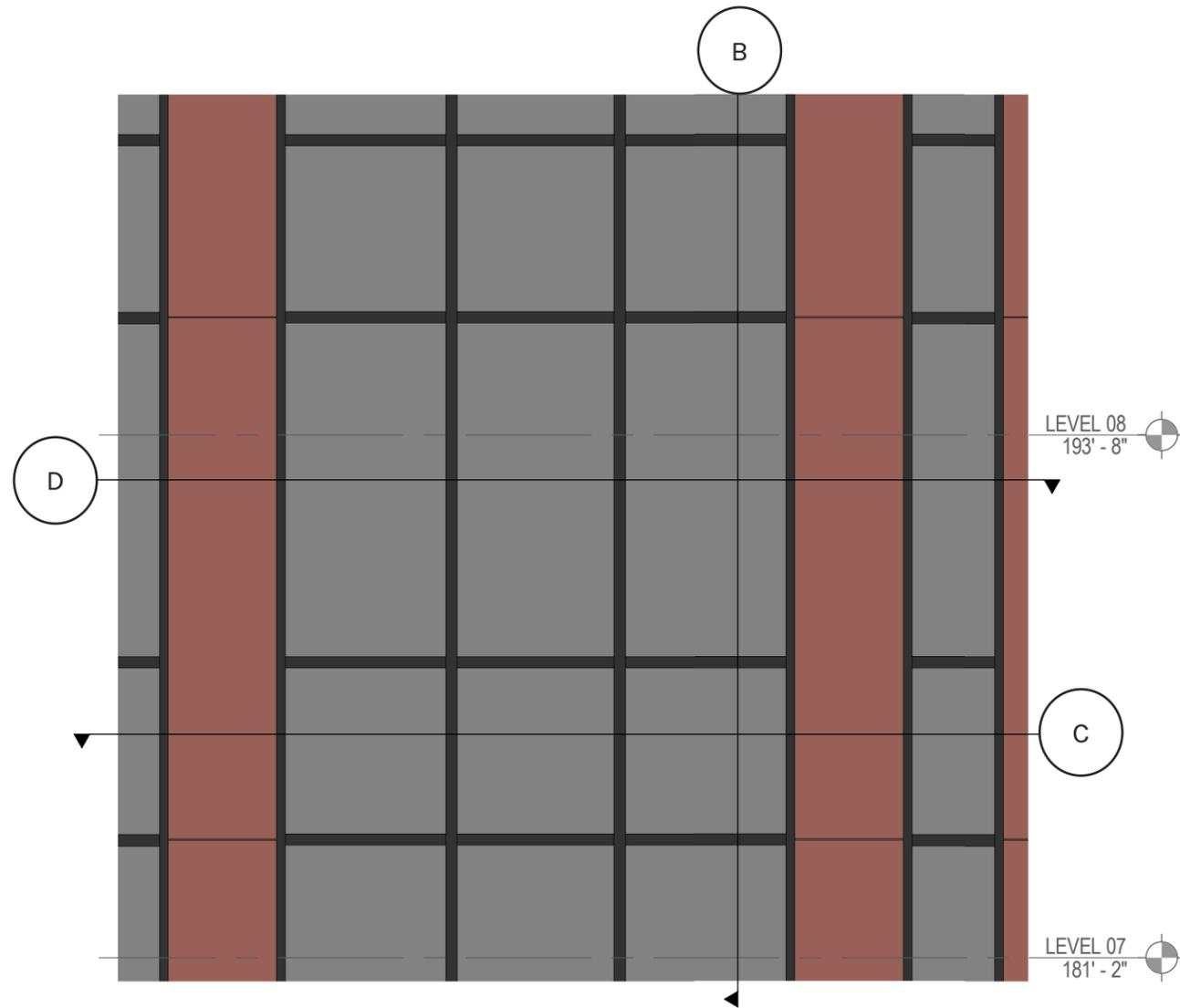
**A** PARTIAL ELEVATION CURTAINWALL - WALL TYPE "C"
