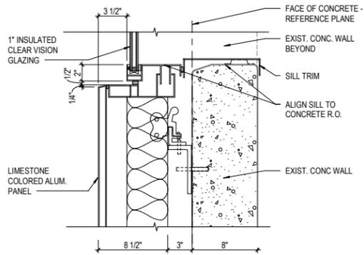
**G** WALL TYPE "B" - SILL AT PUNCHED OPENING
