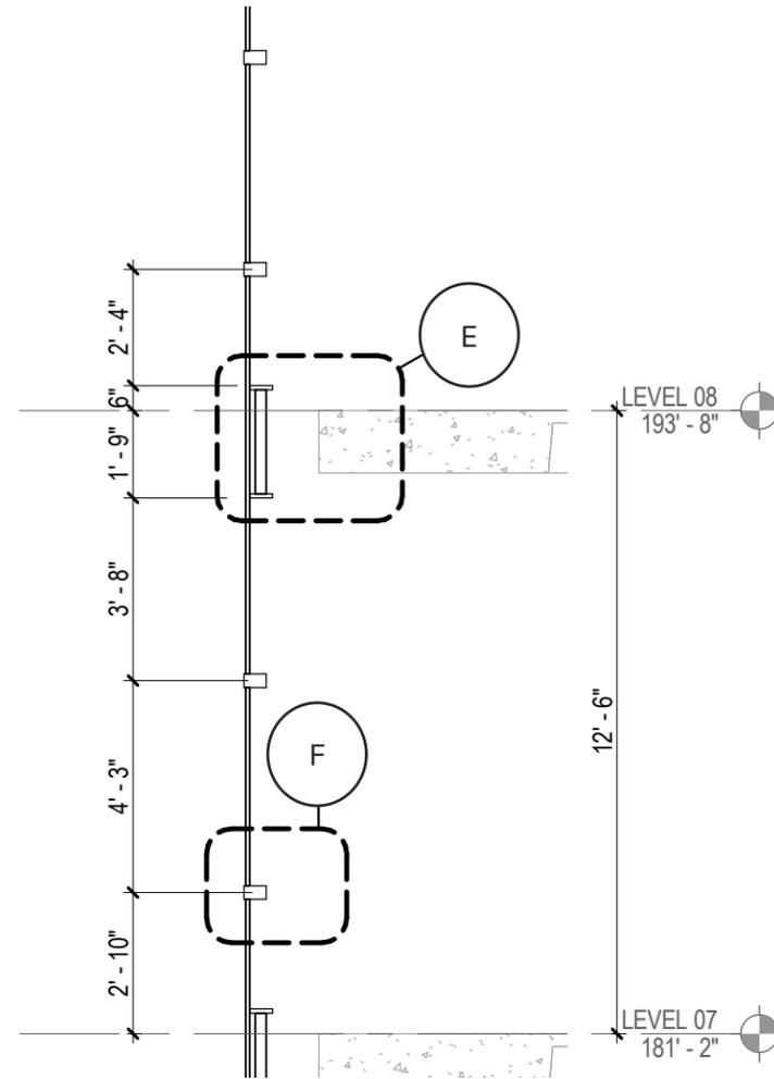
**B** PARTIAL SECTION CURTAINWALL - WALL TYPE "C"
