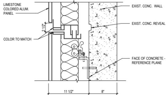
**H** WALL TYPE "B" - STACK JOINT AT REVEAL
