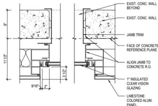
**J** WALL TYPE "B" - JAMB AT PUNCHED OPENING
