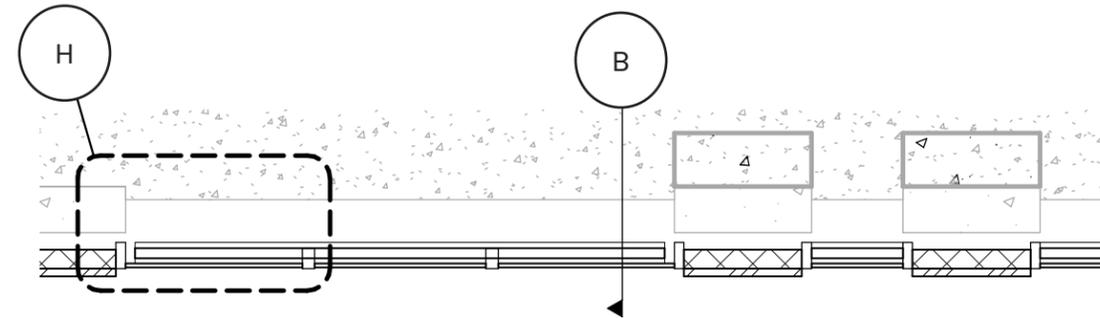
**D** PARTIAL PLAN CURTAINWALL - WALL TYPE "C"
