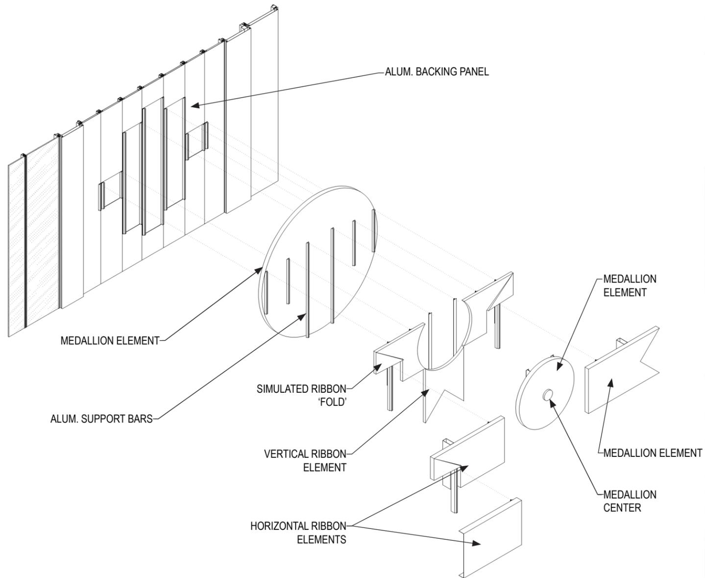
DIAGRAM - EXPLODED ISOMETRIC OF GARLAND ATTACHMENT
