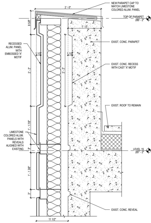
**G** WALL TYPE "B" - PARAPET CONDITION
