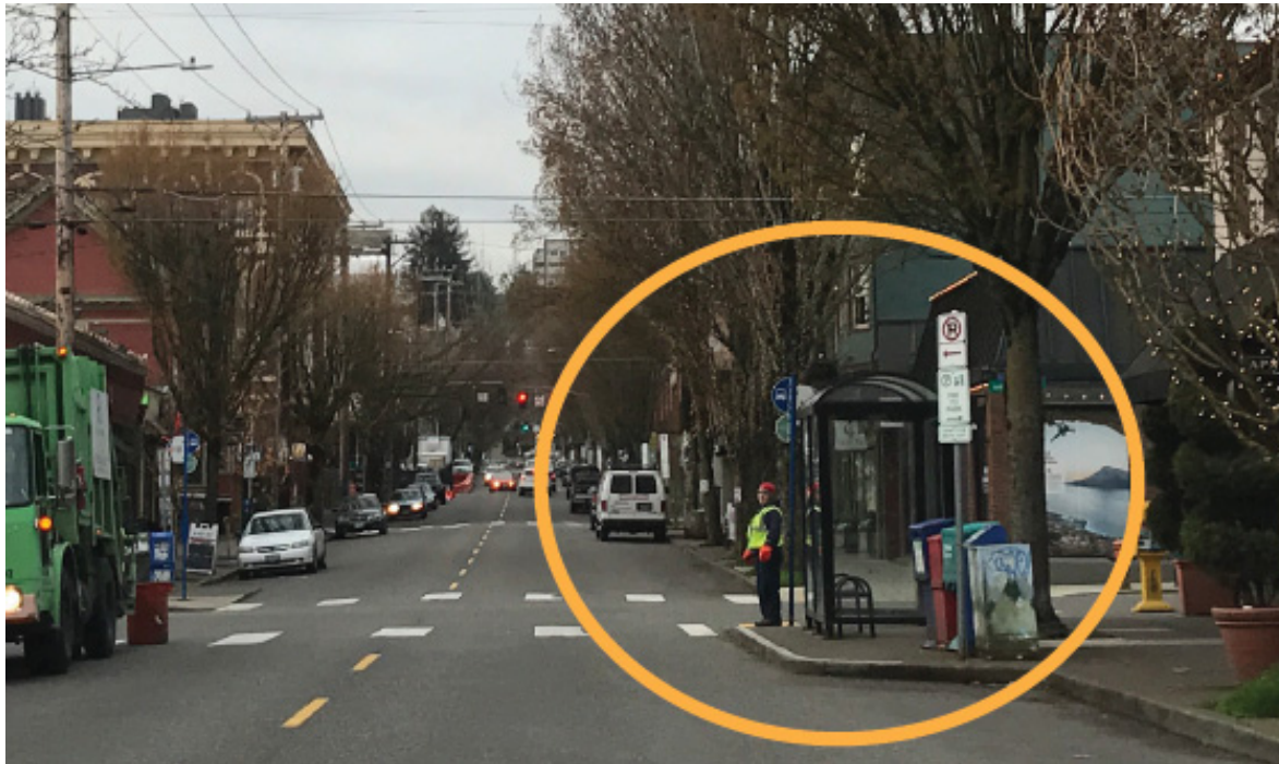
Curb Extension for Stops/Stations
