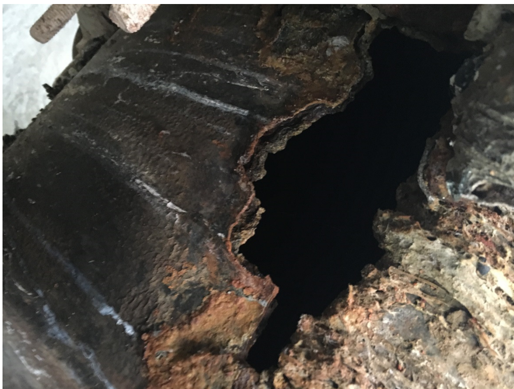
Photo 16 – 2" by 3" hole in east side of Harnessed Mechanical Coupling at Sta. 23+58.
