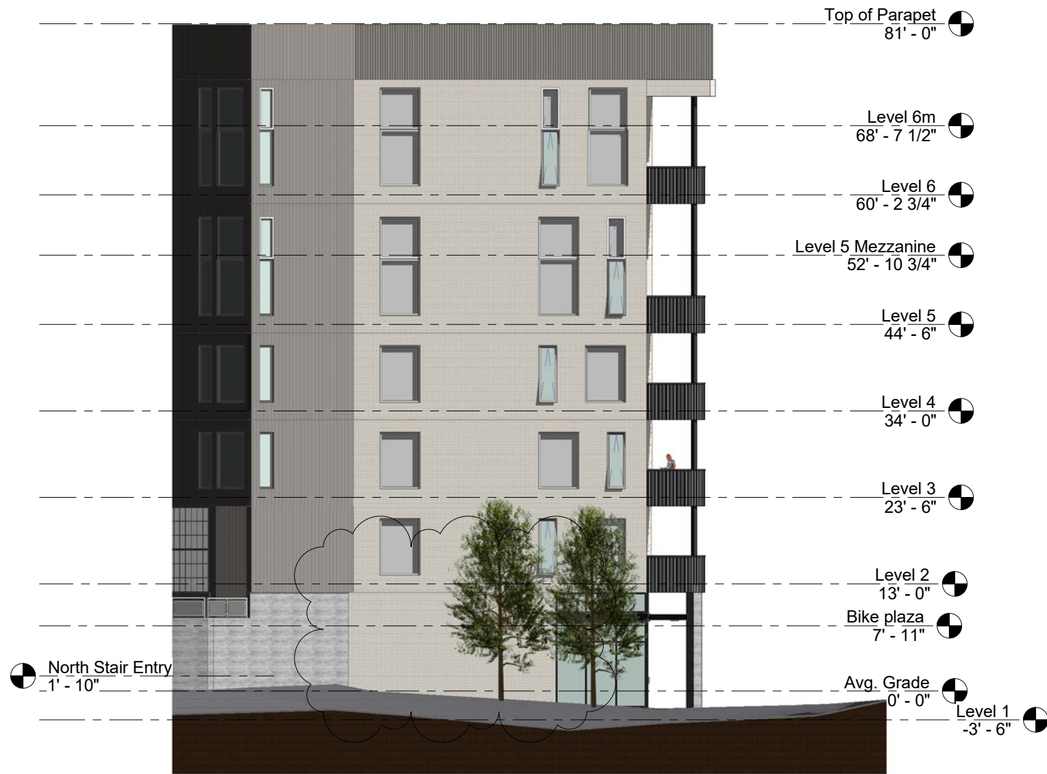
① Elevation at added brick veneer 1/16" = 1'-0"
