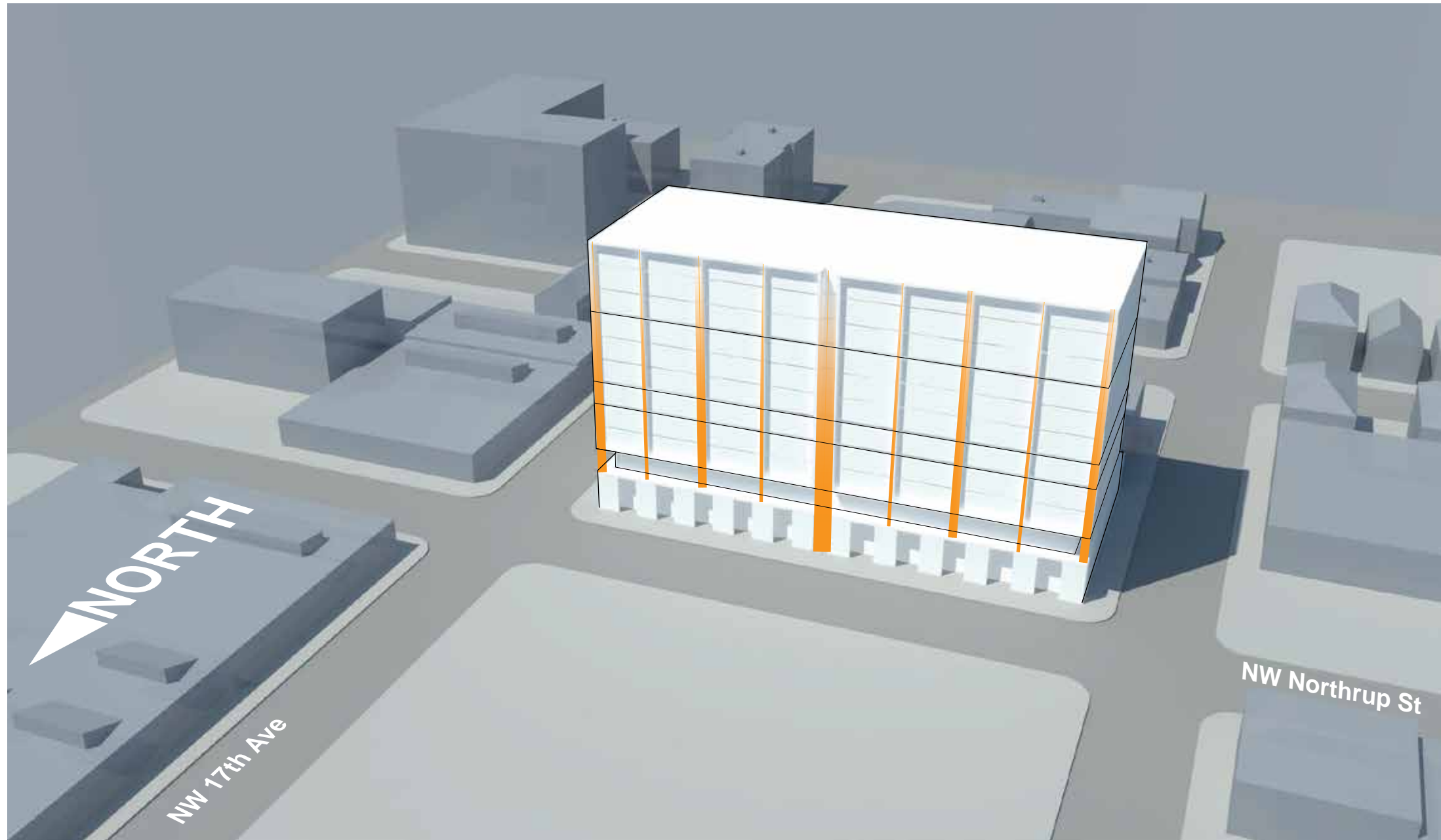
SECONDARY VERTICAL BREAKS (EVERY 25'-50')
