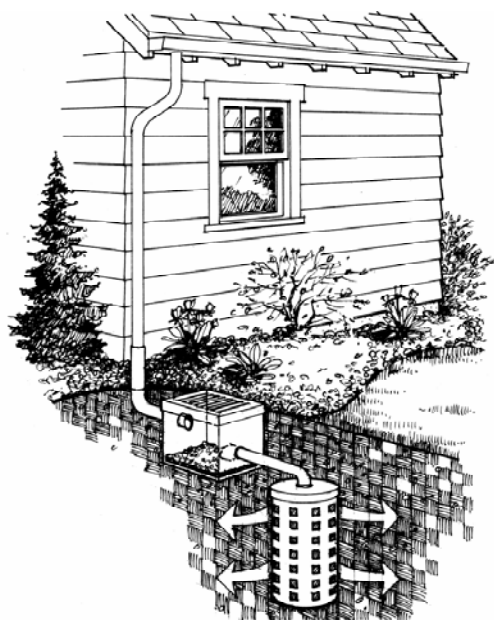
Exhibit 2-30: Drywell illustration. See Appendix G.1 SW-170 for typical drywell details.
