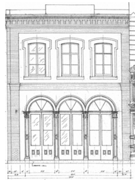
The design for the cast iron façade reconstruction of the Hallock & McMillan Building relied heavily on historic photos taken before incompatible façade changes were made in the 1940s.
