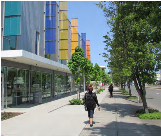
Example of a front setback along a wide Civic Corridor, providing additional space for pedestrians and trees.
