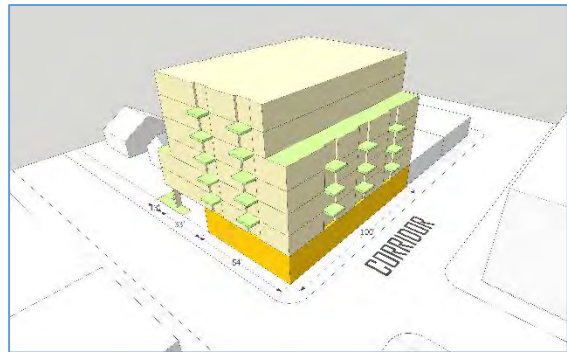
The diagrams above show an example of the massing of development allowances in the CM3 zone. The left diagram shows the maximum base development allowance; the right diagram shows the maximum allowance with bonus.
