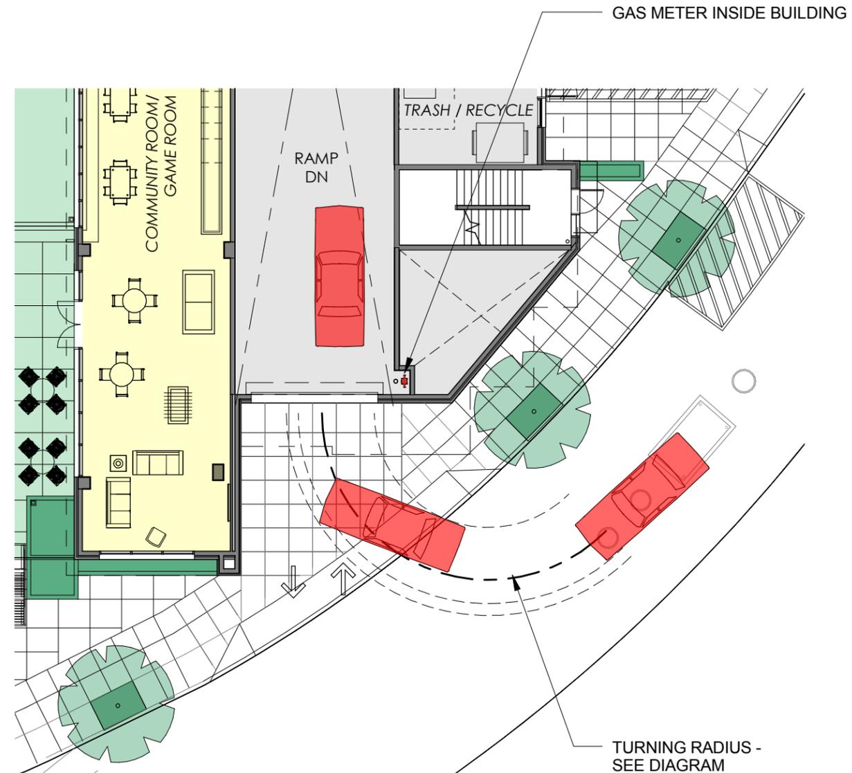
Exhibit 2-3. Minimum Turning Path for Passenger Car (P) Design Vehicle
