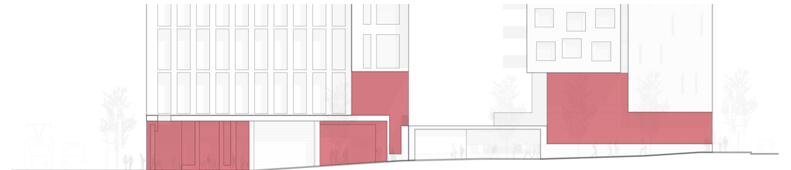
NW Irving Street Elevation: Glazed volumes at intersections and as frames for the Bud Clark Commons courtyard
