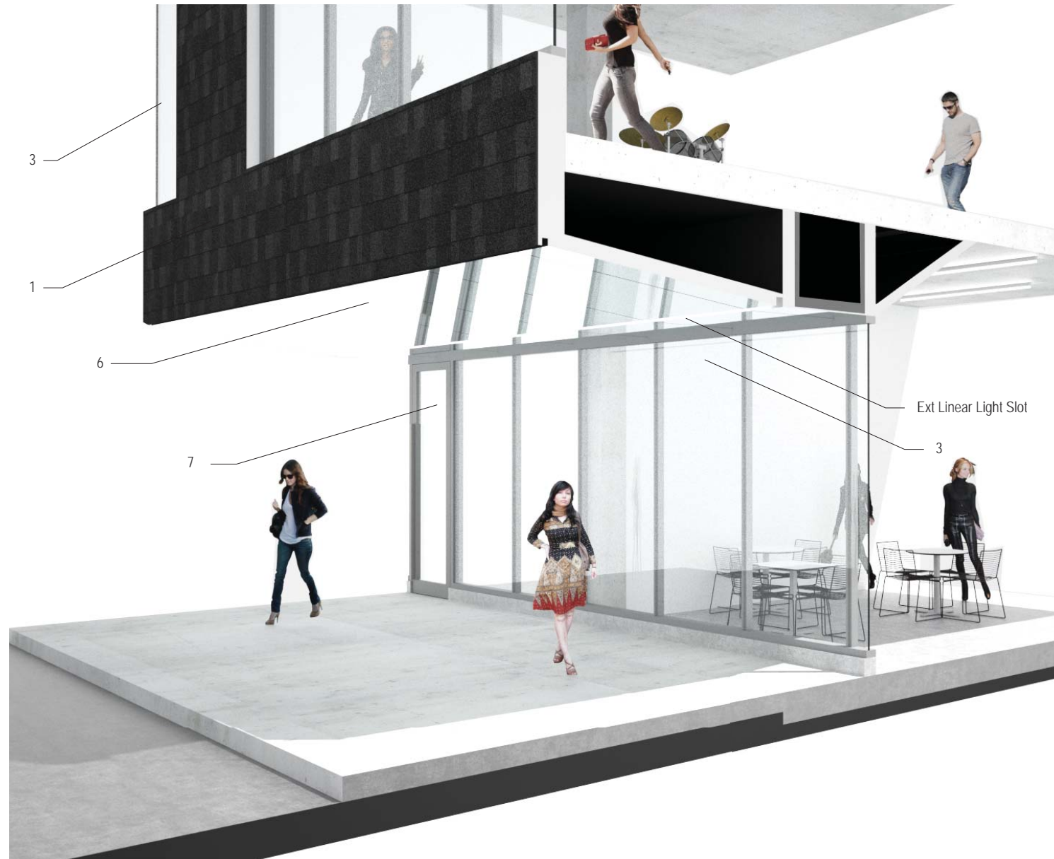
Section of Typical Storefront - E Burnside Street
