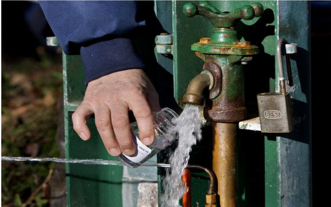
Unacceptable water sampling procedure used by the Portland Water Bureau. Sample should be rejected as there is high contamination risk due to no gloves as barrier and water stream splash
