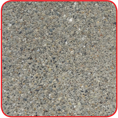
C.I.P. CONCRETE PAVING TYPE 2 EXPOSED AGGREGATE FINISH INTEGRAL COLOR: 100% SANDSTONE GREY GRANITE AGGREGATE
