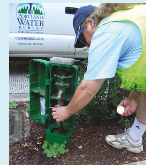
The Portland Water Bureau has 184 water quality sampling stations throughout the distribution system to monitor water quality on a regular basis.
