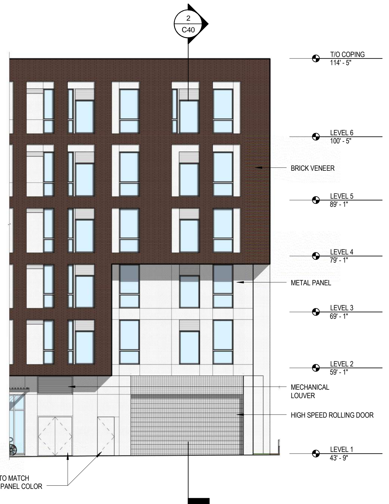
ENLARGED WEST ELEVATION ①
