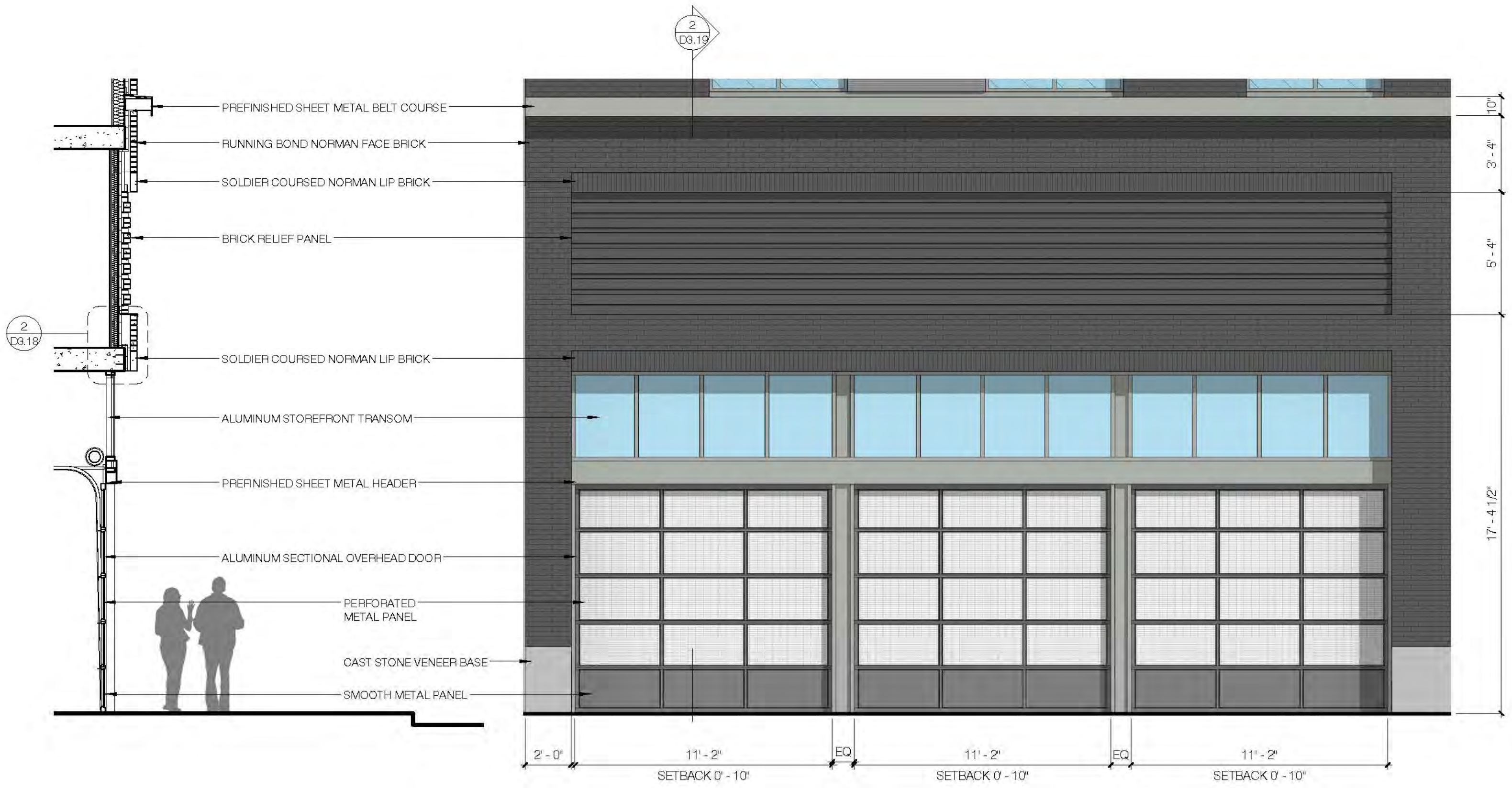
2 WALL SECTION@ PARKING ENTRY 1/4" = 1'-0"
