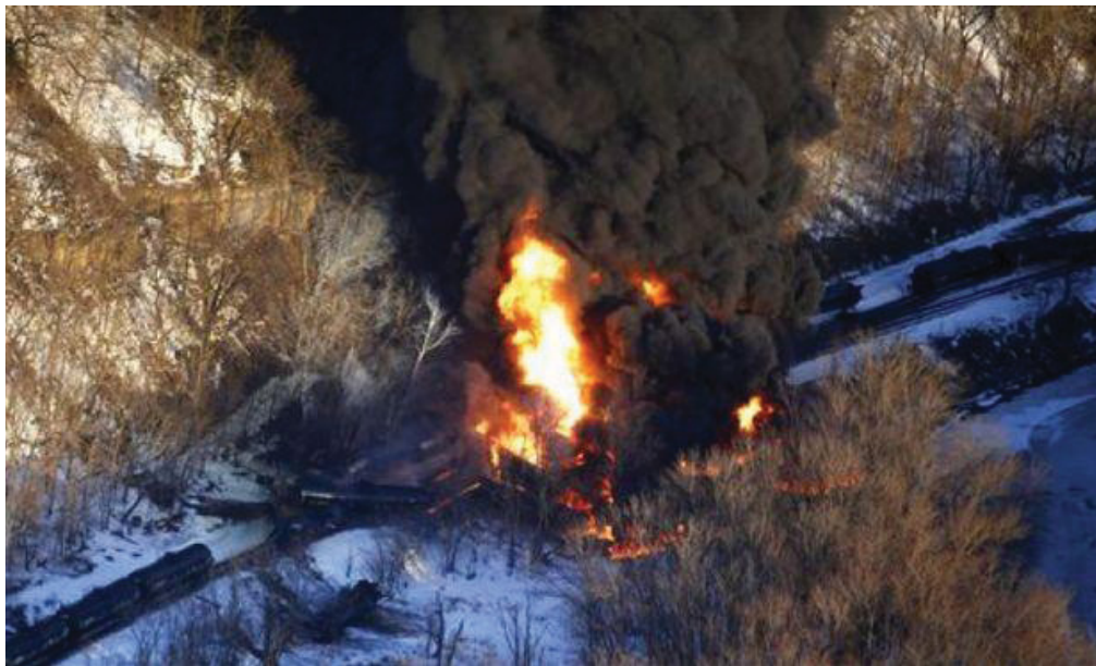
Smoke and flames erupt from the scene of a train derailment Thursday, March 5, 2015, near Galena, IL. A BNSF Railway freight train loaded with Bakken crude oil derailed 21 tanker cars around 1:20 p.m. Two cars split open, burned, and set fire to three others cars, in a rural area where the Galena River meets the Mississippi. The tanker cars were the "newly improved" DOT-111/CPC-1232 type (AP Photo/Telegraph Herald, Jessica Reilly)
