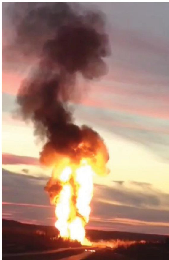
DOT112J propane tanker derailment, belly breach, cold BLEVE and fireball, near Gainford, Alberta, Oct 19, 2013. The Canadian TSB investigation report R13E0142 (Published Feb 24, 2015) cites critical design faults in DOT112J340W. The NWCSI
