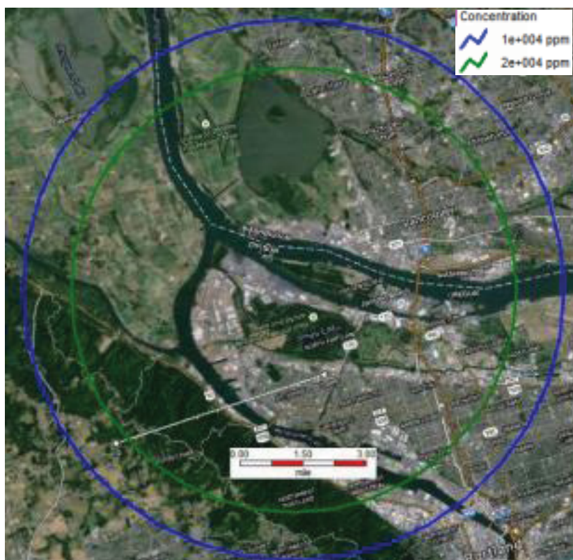
Figure 4-2 Worst-Case Release Scenario, LPG Storage Tank, Flammable Dispersion Effect Zones (360deg rotation of potential cloud plume)
