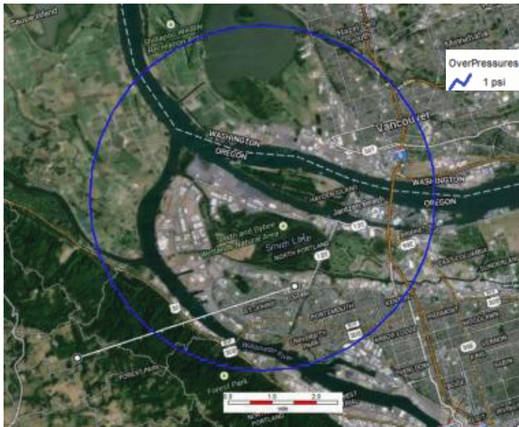
Figure 4-1 EPA RMP Worst-Case Release Scenario, LPG Storage Tank, 1 psi Overpressure Effect Zone
