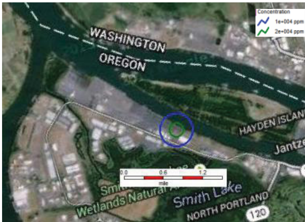
Figure 3-3 Instantaneous Release Scenario, Pressure Storage Vessel, Flammable Dispersion Effect Zones (360 deg rotation of potential cloud plume)
