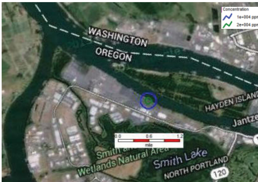
Figure 4-4 Worst-Case Release Scenario, Railcar, Flammable Dispersion Effect Zones (360 deg rotation of potential cloud plume)
