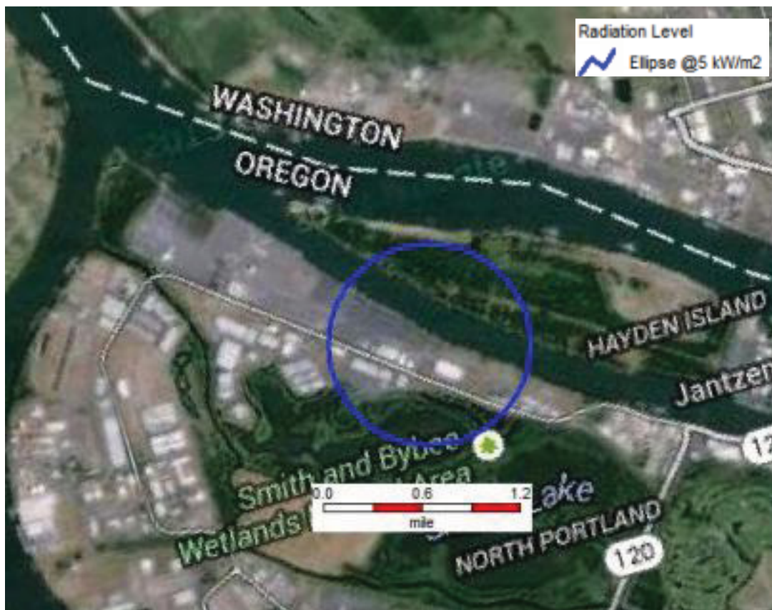
Figure 3-4 BLEVE, Pressure Storage Vessel, 5 kW/m 2 Thermal Radiation Effect Zone
