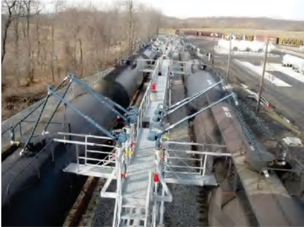
Figure I-19: Rail Car Offloading Arrangement (Ref. 3)
