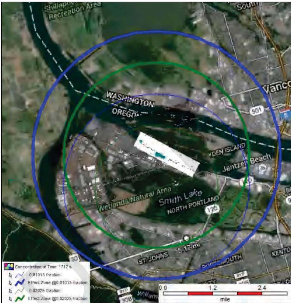
Figure III-5: Worst Flammable Dispersion Effect Zones at 1 m (3.3 ft) Elevation above the ground for Catastrophic Rupture of Storage Tank 1 (S04-01C-R3), F 1.8 m/s (4.0 mph) Summer-Night Weather Condition
