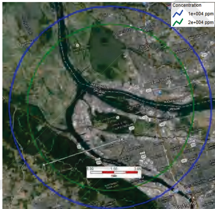
Figure 4-2 Worst-Case Release Scenario, LPG Storage Tank, Flammable Dispersion Effect Zones (360deg rotation of potential cloud plume)
