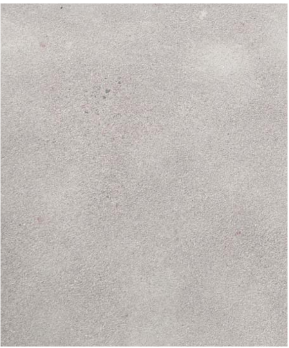
enhanced concrete paving poured-in-place concrete paving with integral color and decorative aggregate with acid etch or light sandblast finish application.
