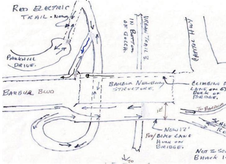
The sketch above shows how the connection from SW Parkhill will connect to the Newbury Bridge. The photo below illustrates the same concept.
