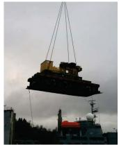
The Dredge Oregon went to dry dock in November 2012 for Phase I of the repower project. An opening was cut out of the hull of the vessel to remove the large, WWII era auxiliary engine and replace it with a smaller more efficient engine that meets EPA Tier III emissions standards.
