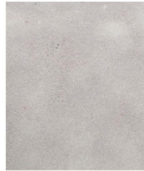
enhanced concrete paving poured-in-place concrete paving with integral color and decorative aggregate with acid etch or light sandblast finish application.
