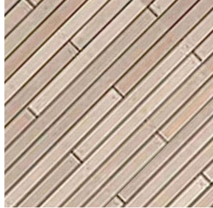
Okoskin (147 mm, sandstone, 45 deg angle, hat channel furring max 24" o/c)
