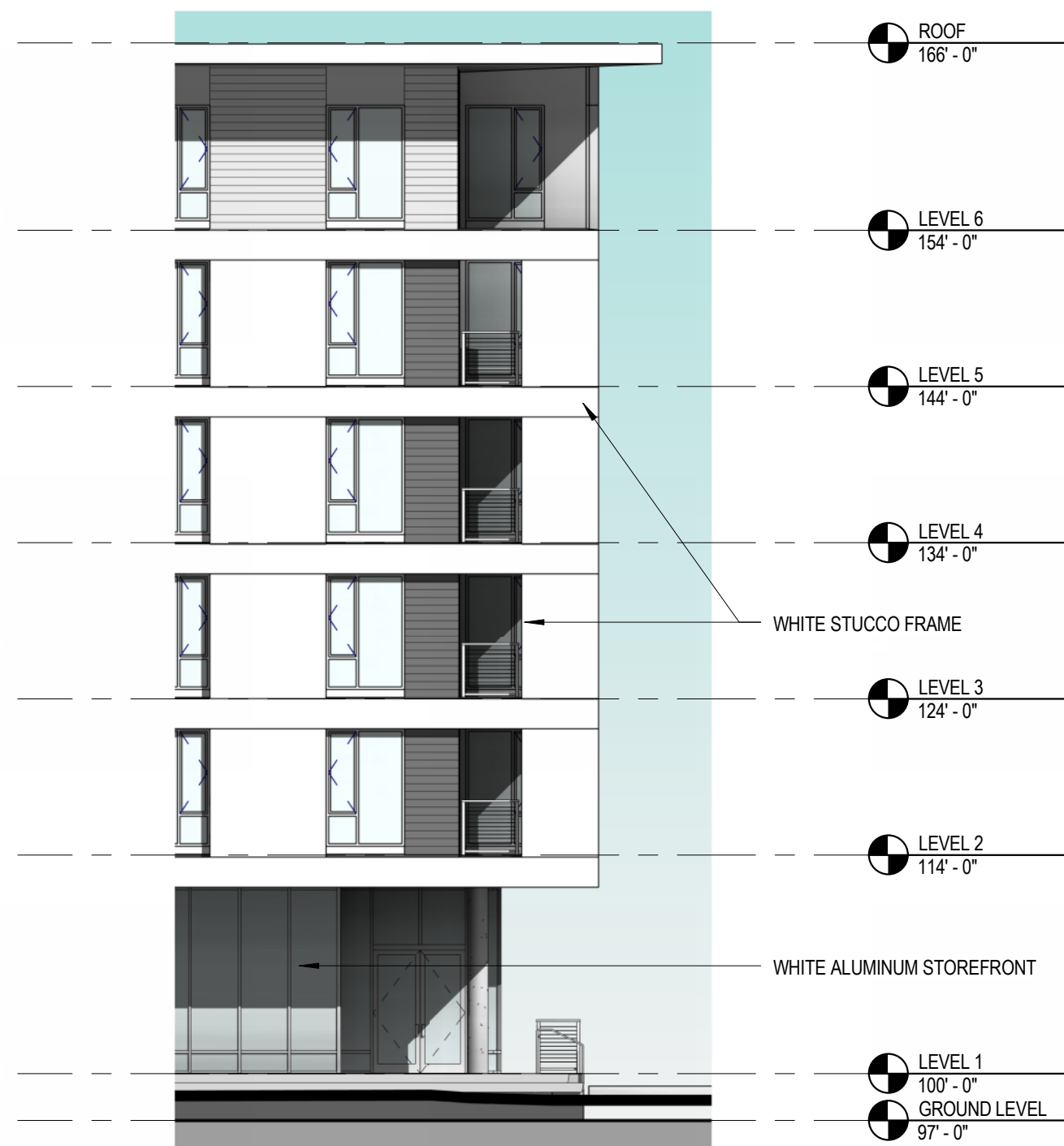
BUILDING A - ENLARGED WEST ELEVATION ①
