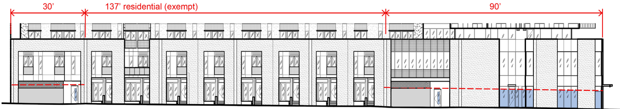
NW PETTYGROVE ELEVATION total glazing length: 25'-0" (20.8%) total glazing area: 235 sq ft (18.5%) applicable facade: 120'-0" length; 1,270 sq ft area
