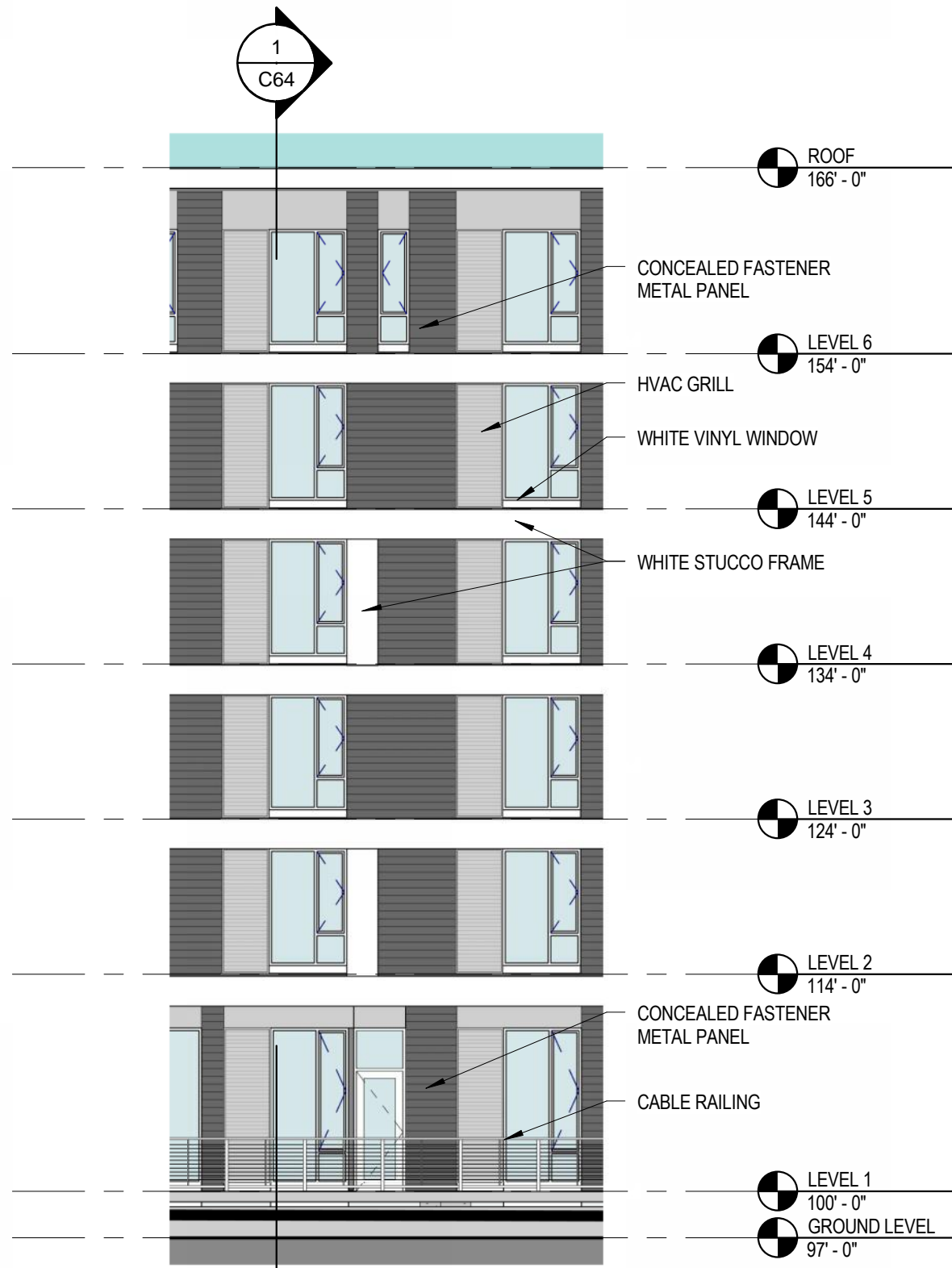
BUILDING A - TYPICAL ENLARGED ELEVATION ②
