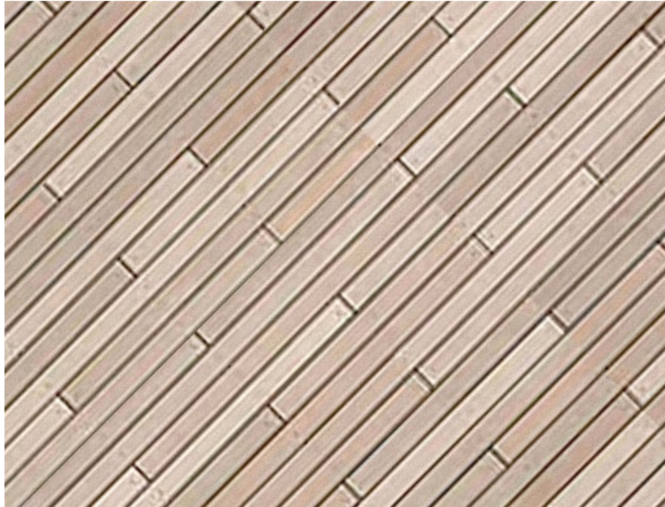
Okoskin (147 mm, sandstone, 45 deg angle, hat channel furring max 24" o/c)
