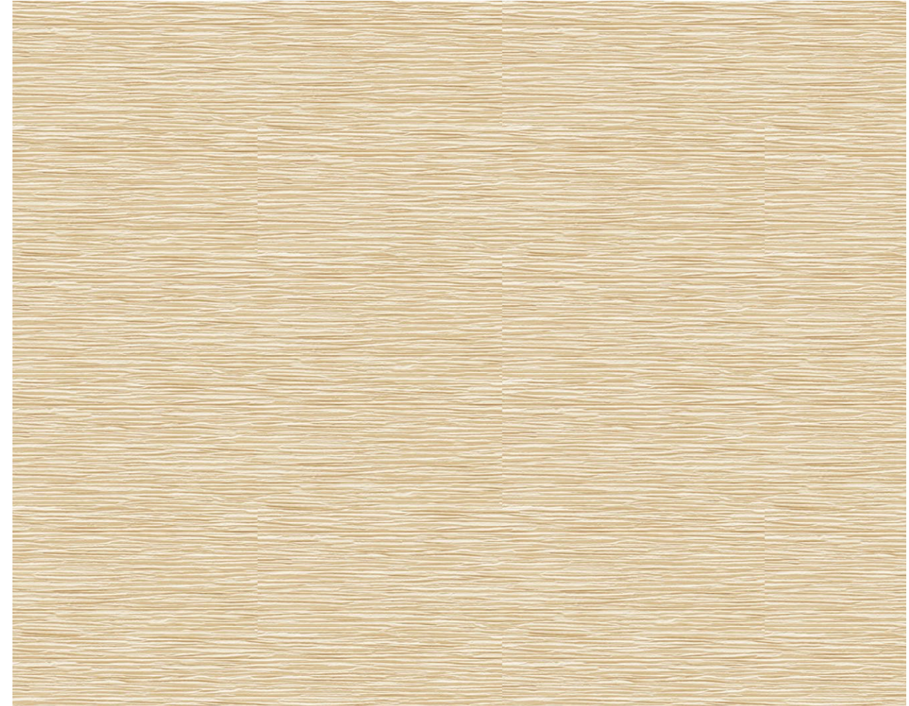
Ceraclad (Fiotto, vanilla, 18" horizontal, hat channel furring max 16" o/c)
