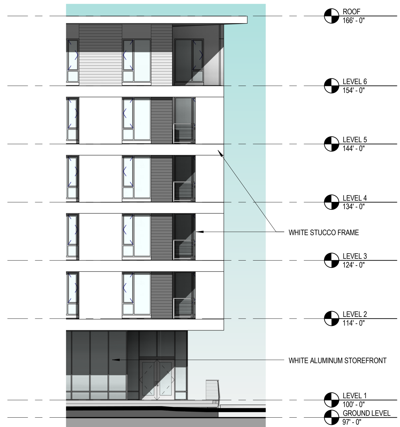
BUILDING A - ENLARGED WEST ELEVATION ①
