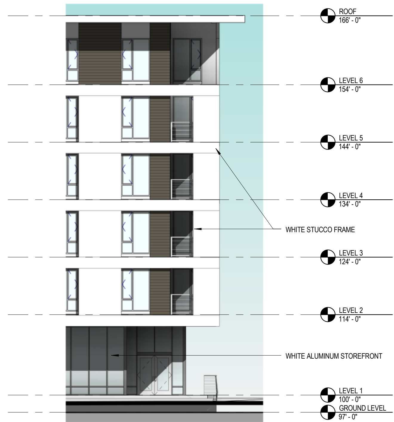
BUILDING A - ENLARGED WEST ELEVATION ①
