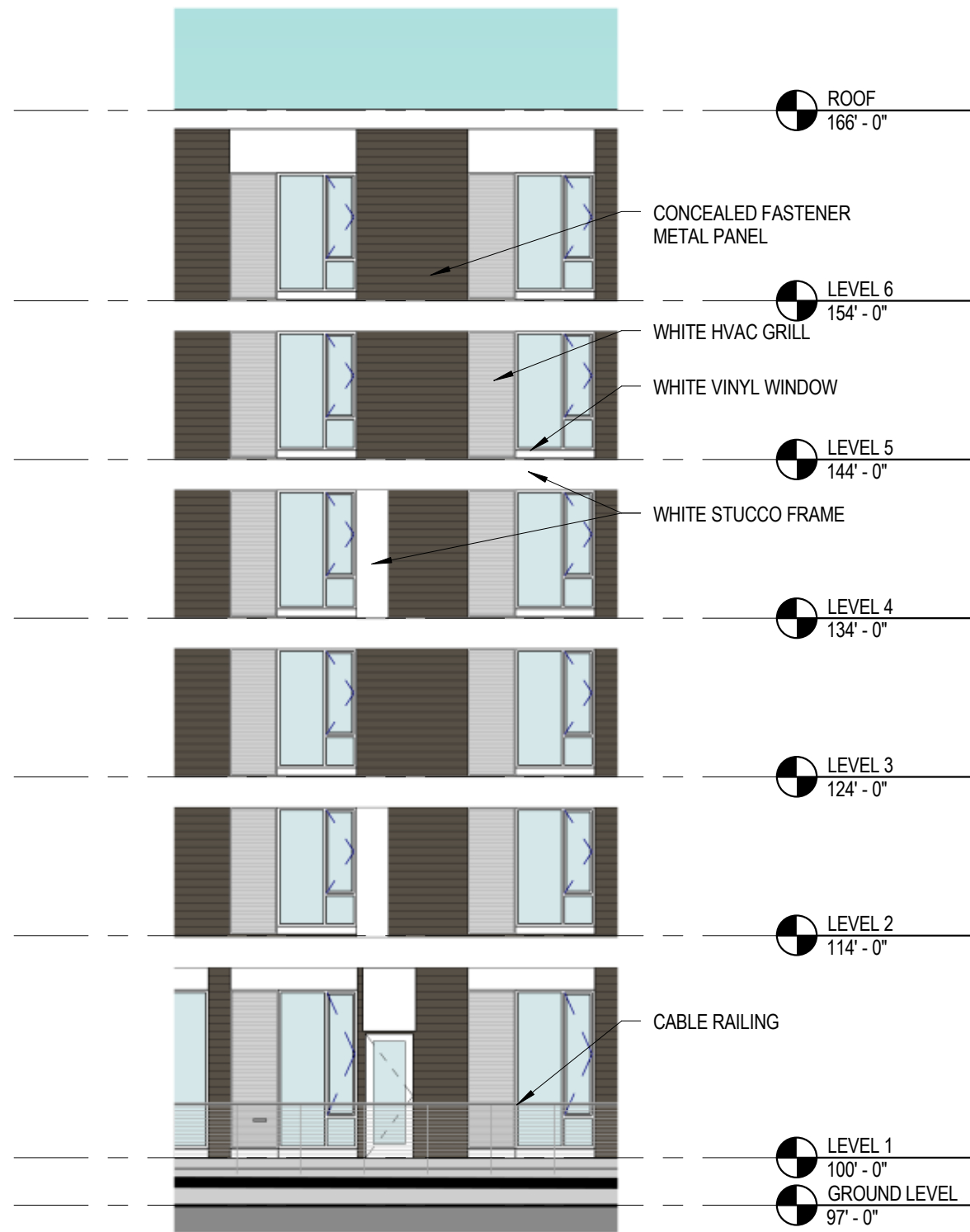
BUILDING A - TYPICAL ENLARGED ELEVATION ②
