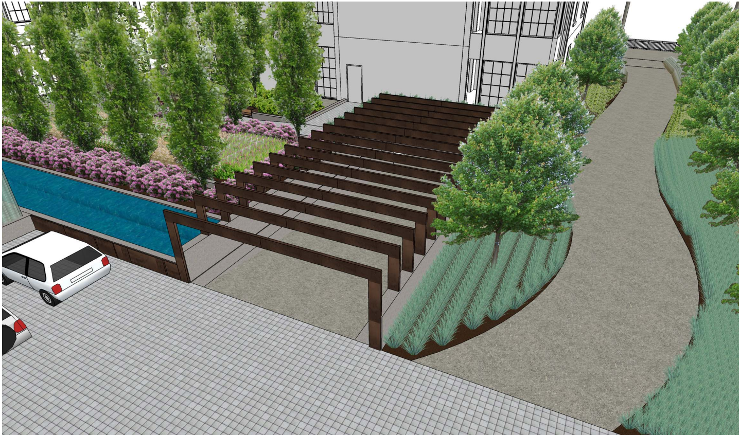
Metal structure above garage ramp
