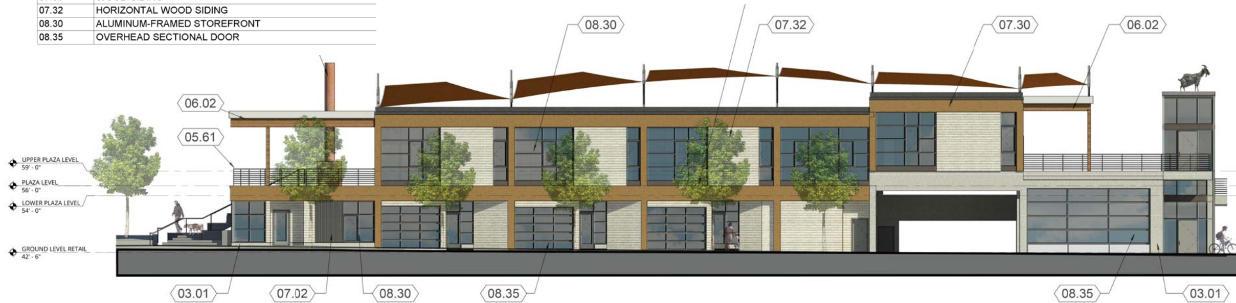
Elevation - West 1"=20'-0" Elevation
