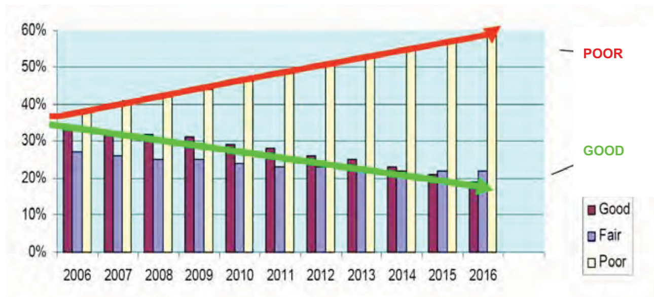
Figure 8.17 Projection of Pavement Condition, 2006 to 2016
