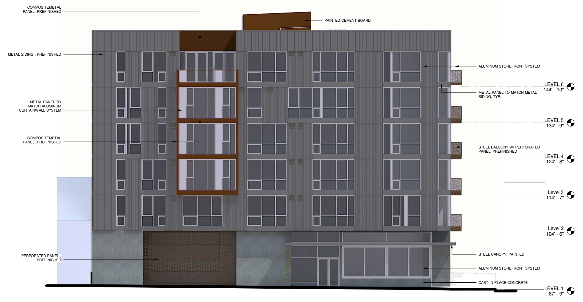
① EXTERIOR ELEVATION FACING EAST 1/8" = 1'-0"
