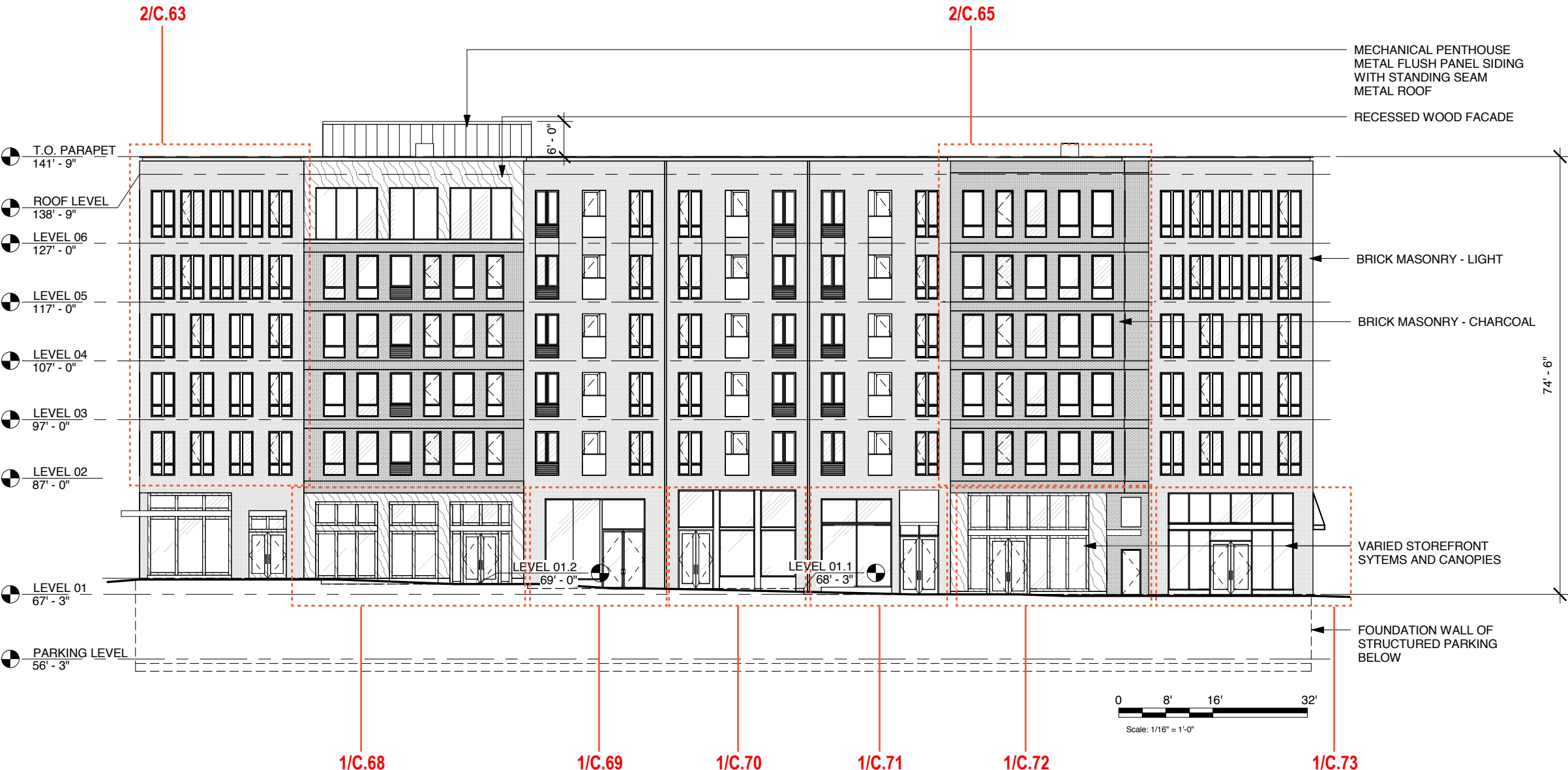
C.55 East Building Elevation
