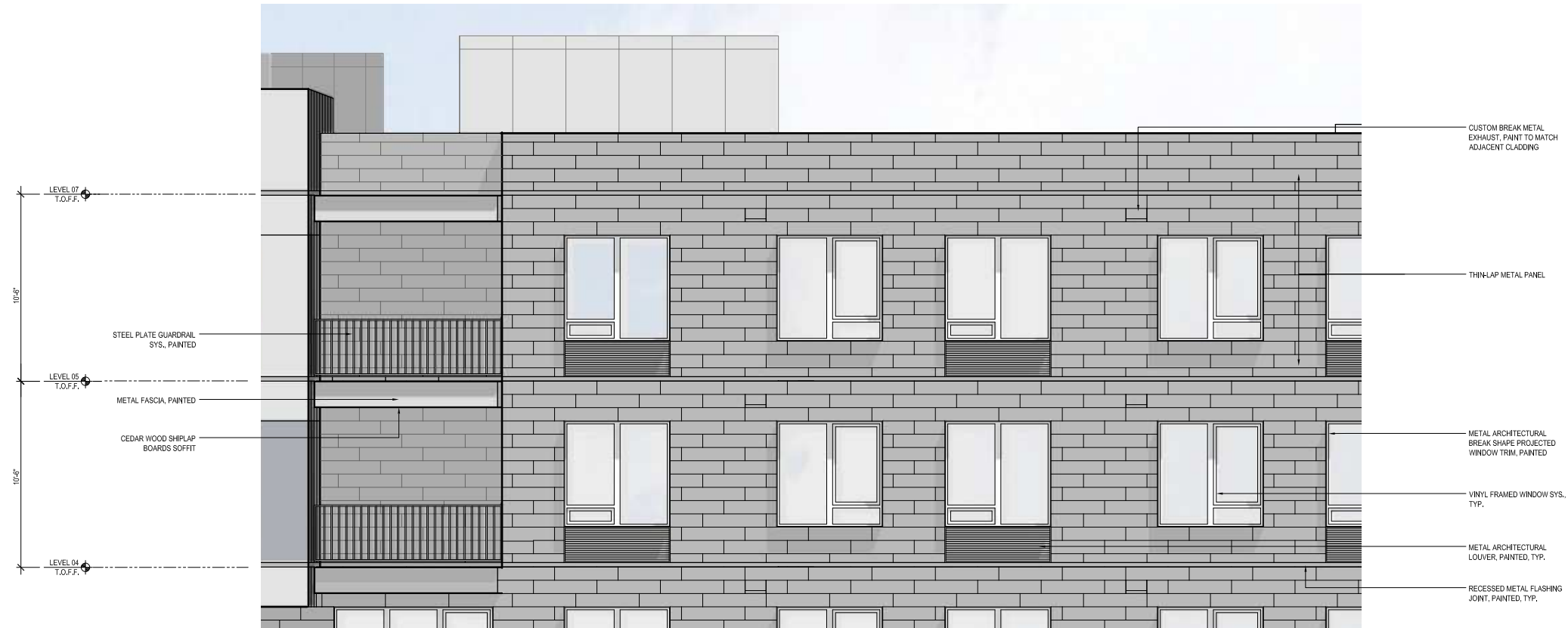
1. ENLARGED PARTIAL EXTERIOR ELEVATION - SOUTHWEST, TYPICAL
