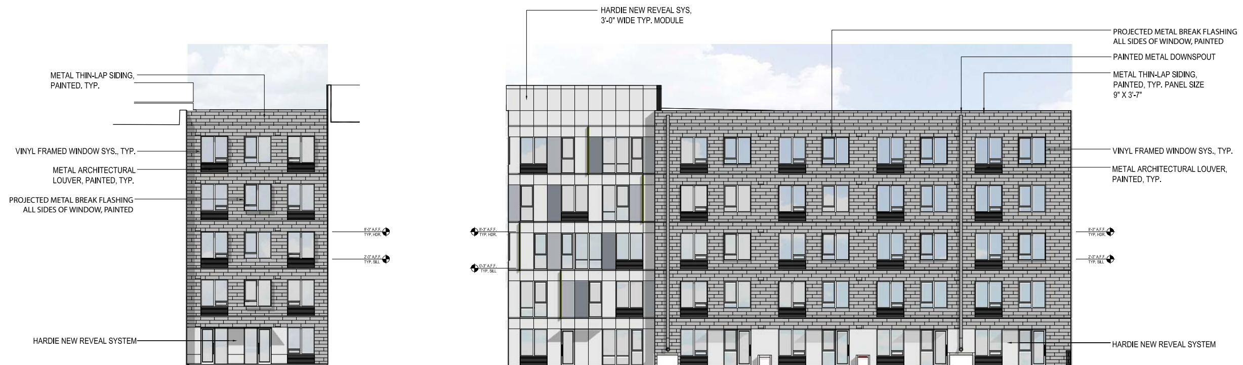
1. ELEVATION - SOUTH COURTYARD
