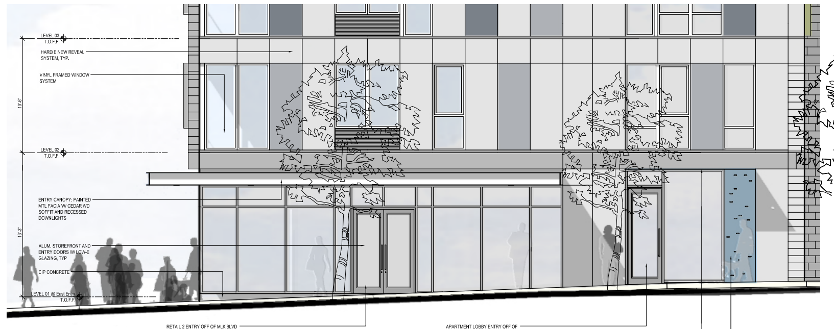
1. ENLARGED PARTIAL EXTERIOR ELEVATION - EAST ENTRY
