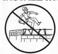
DO NOT walk on the joists until all joist bearings and bracing attached. Injury may result
