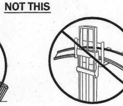
DO NOT lift joists in the flat orientation
