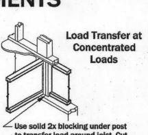
to transfer load around joist. Cut blocks 1/16" longer than joist depth.
