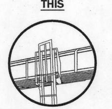
Lift joists from underside only. DO NOT dump or drop from truck.
