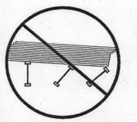
DO NOT stack building joists. Stack only over
