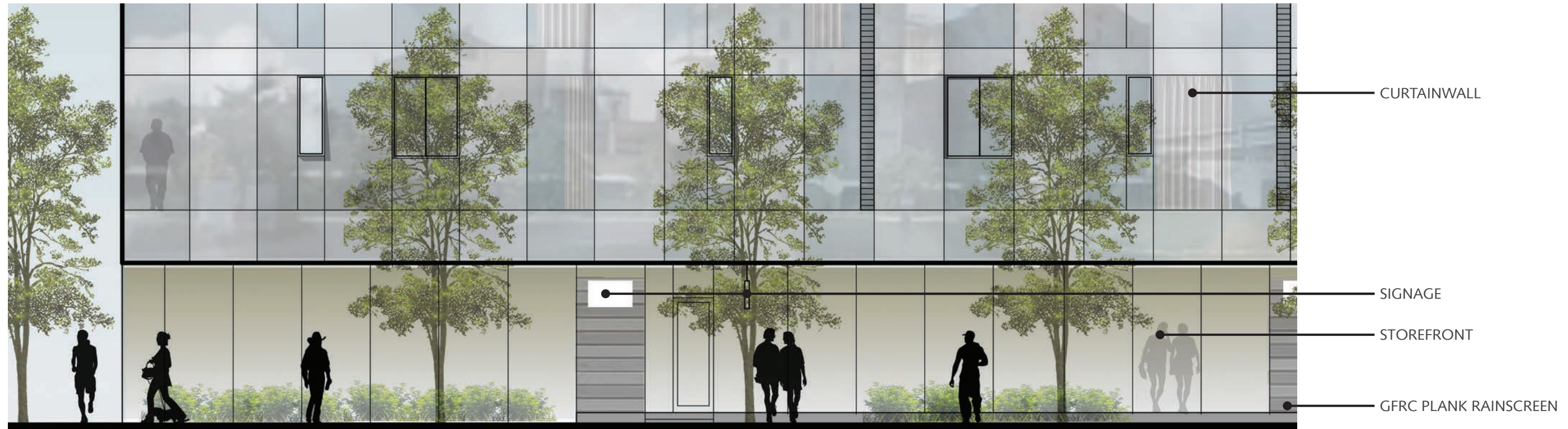
Enlarged Street Level Elevation - North Elevation @ Lobby
