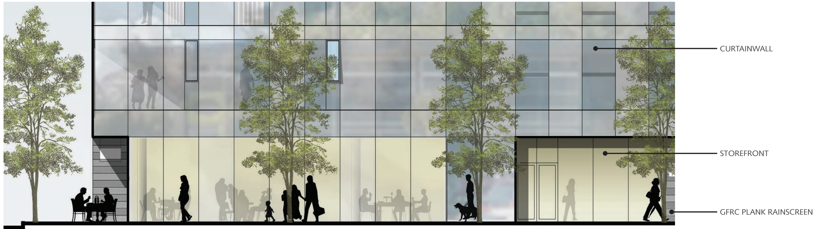
Enlarged Street Level Elevation - East Elevation @ Retail
