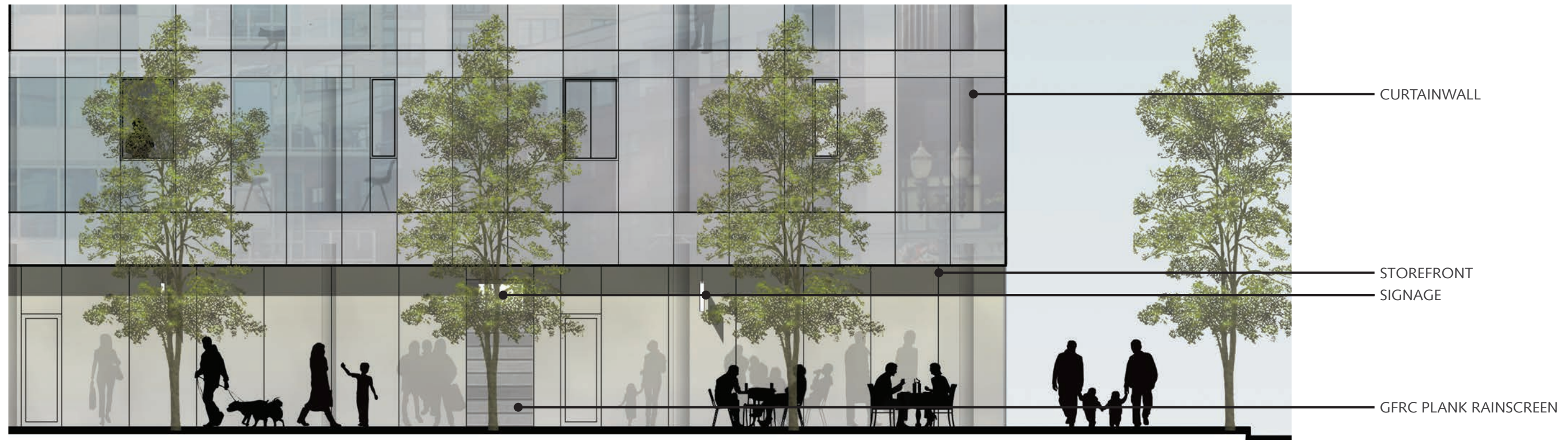
Enlarged Street Level Elevation - South Elevation @ Retail
